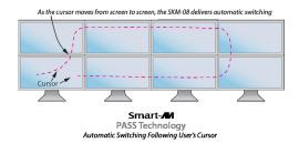
\*PASS does not work in Multi-head display mode.
